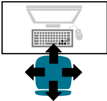
Figure 3. Frequently used music player commands are mapped to the four canonical directions.
